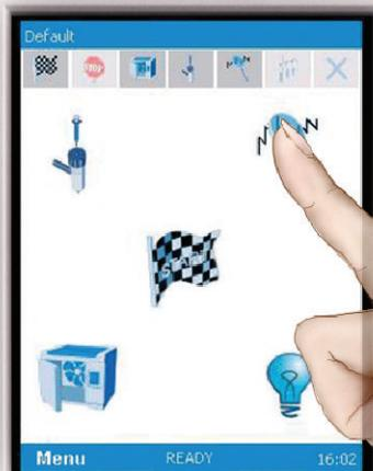
Unlike other commercially available fast gas chromatographs, the MASTER GC offers guided diagnostics and maintenance procedures supporting the user in the preservation of the systems precision. The outcomes can be monitored and controlled through the touchscreen display.
